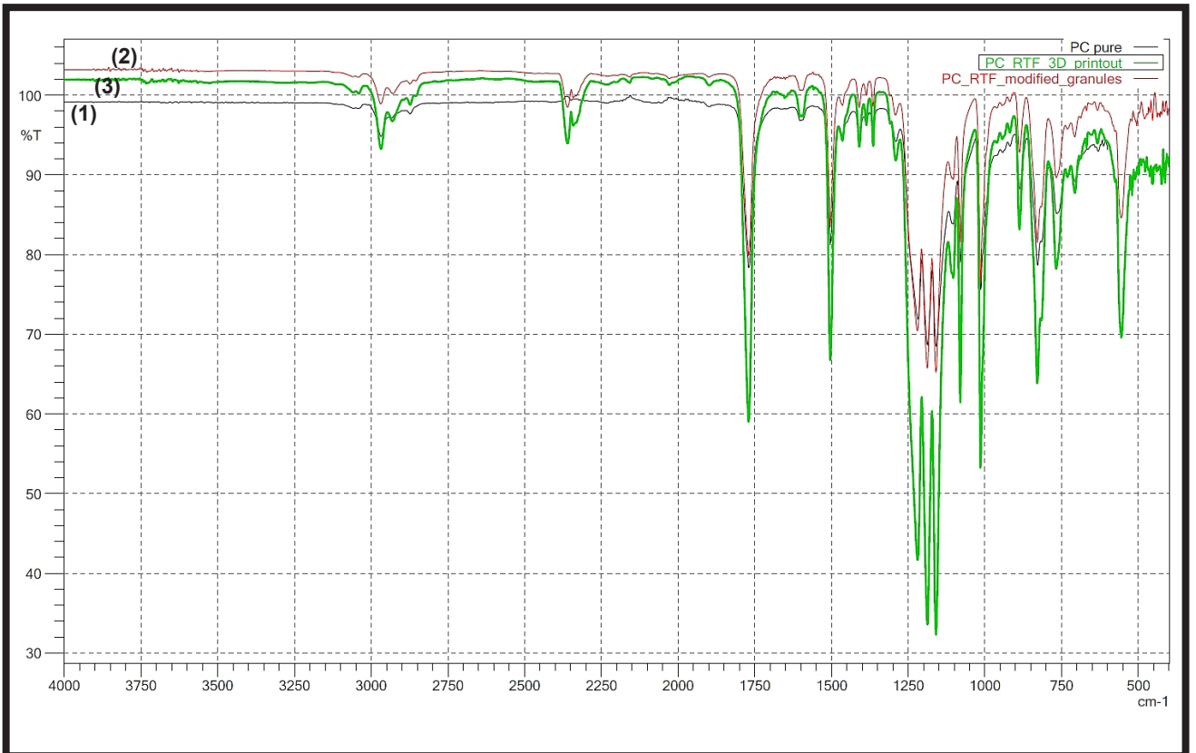
FIG. 5. Evolution of the IR spectra during thermal processing of the composite compared with pure polycarbonate. PC – black (1), modified granules – red (3), modified material printout from 3D printer – green (2).
