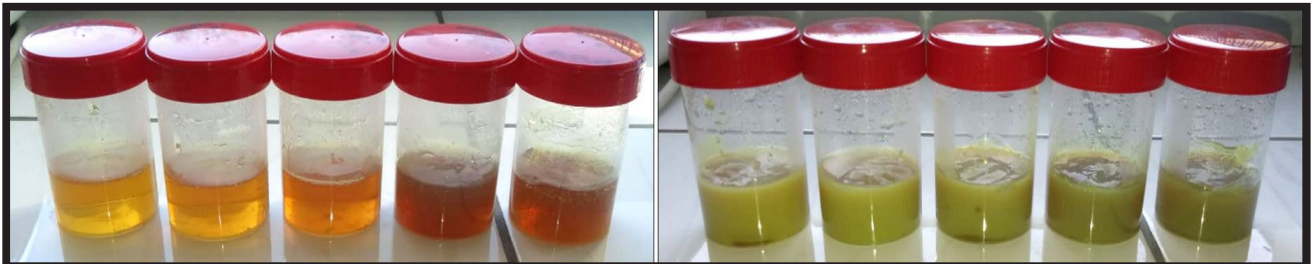
FIG. 2. The obtained samples before (left) and after (right) the single crosslinking, according to increasing mass ratio of VAN:CS.
