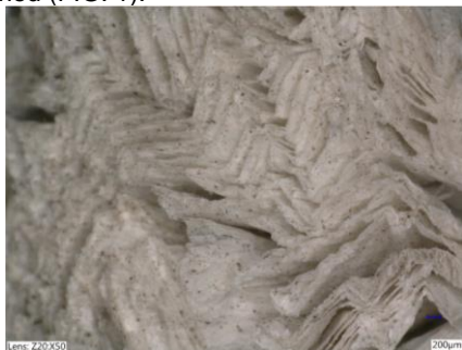
FIG. 1. Digital microscope image of freeze-dried 1CS_1GEL_1PVA_GO_HAp sample.
