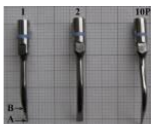
Fig.1 Design of the tips chosen for the study. The free end of the tip is placed parallel to the biofilm during the disruption. The threaded end of the tip is attached to a handpiece.
