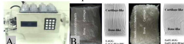
Figure1. A: Rotational Dual Chamber Bioreactor prototype [3]; B: Bilayered structures of LAGG-LAGG/HAp30% (left) and LAGG/Gelatin-LAGG/Gelatin/HAp30% (right).
