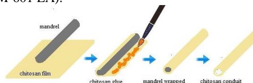
Figure 1 – Scheme of chitosan scaffold fabrication.
