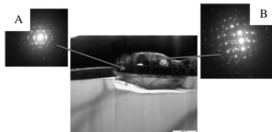
Fig.1. Microstructure and SAED patterns of unmodified (A) and modified (B) channel surface area.
