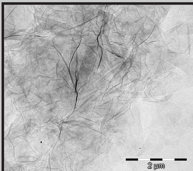
FIG. 3. TEM microphotograph of graphene oxide (GO).
