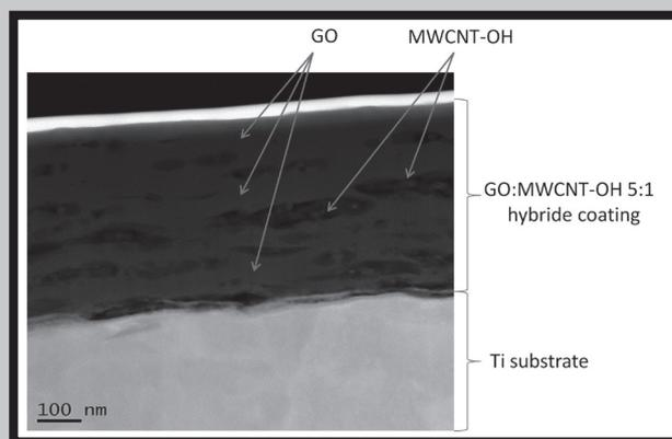
FIG. 10. Microphotograph STEM of GO:MWCNT-OH 5:1 hybrid coating on Ti substrate.
