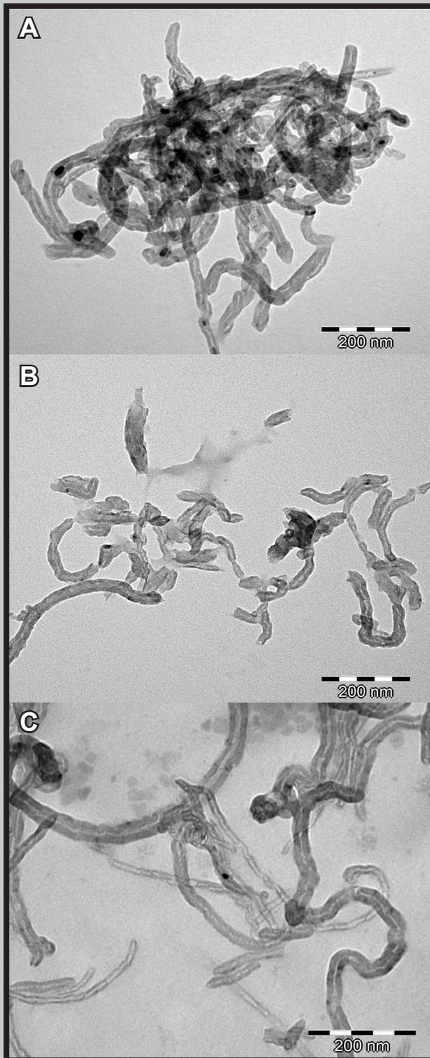
FIG. 4. TEM microphotographs of MWCNT (A), MWCNT-F (B) and MWCNT-OH (C).
