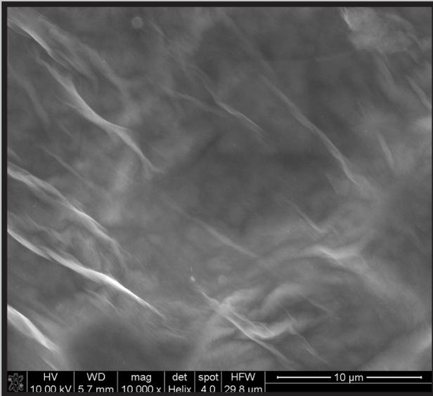
FIG. 6. SEM microphotograph of GO; magnification 10 000x.
