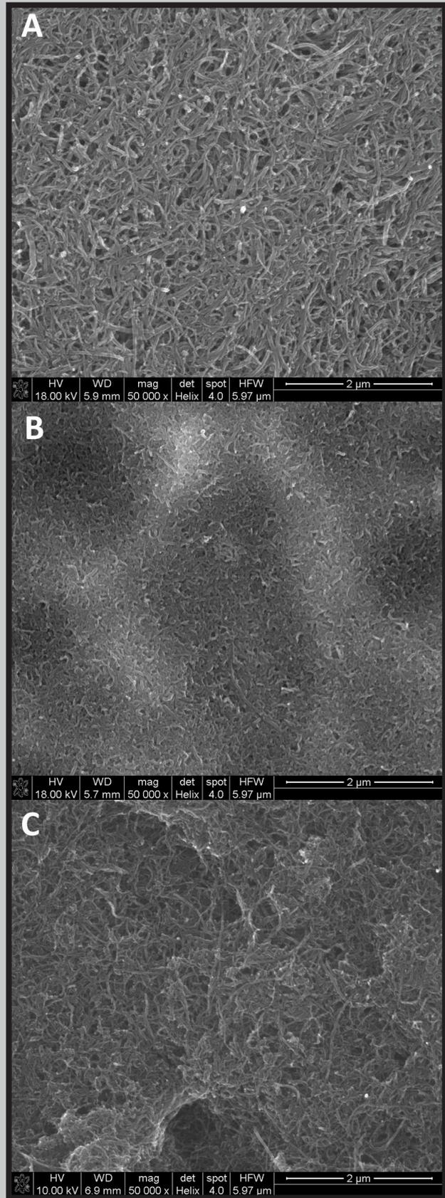
FIG. 7. SEM microphotographs of MWCNT (A), MWCNT-F (B) and MWCNT-OH (C); magnifications 50 000x.
