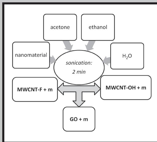
FIG. 1. Preparation of the nanomaterials' suspensions in the mixture of ethanol, acetone and water.
