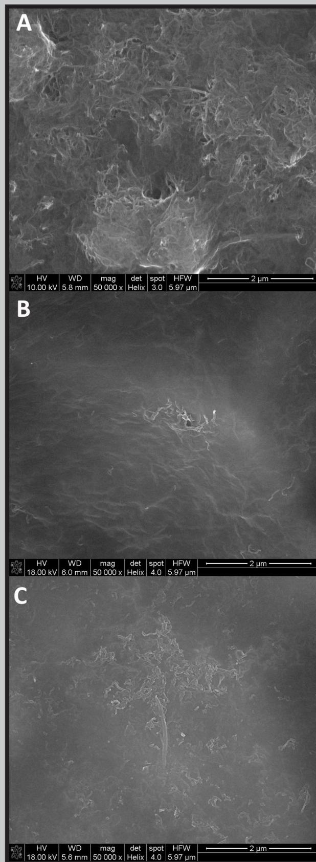
FIG. 8. SEM microphotographs of deposited hybrid layers: GO:MWCNT-OH 1:1 (A); GO:MWCNT-OH 5:1 (B) and GO:MWCNT-F 5:1 (C); magnifications 50 000x.
