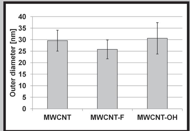
FIG. 5. Average outer diameters of all three types of carbon nanotubes.
