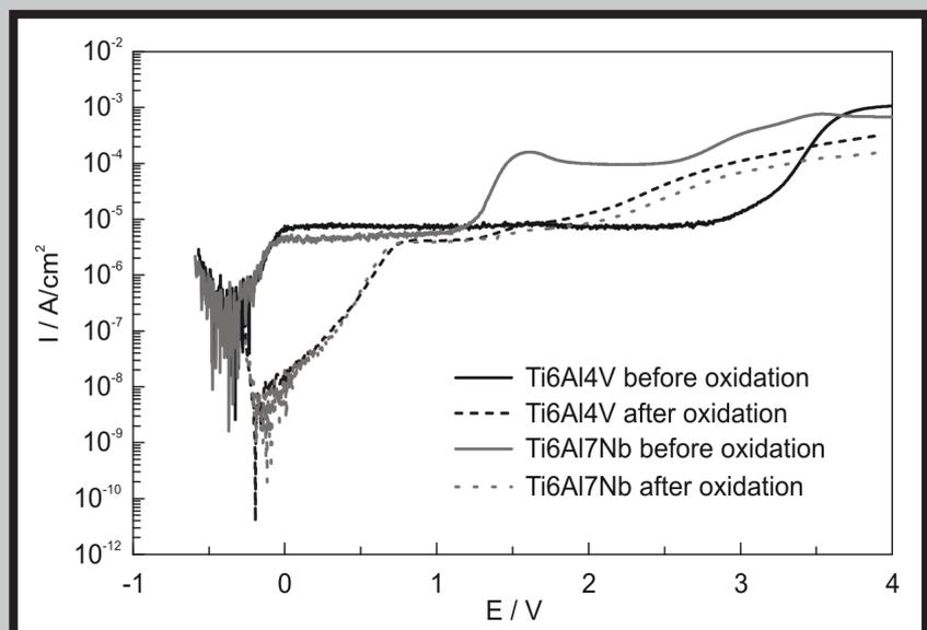
FIG. 5. Potentiodynamic characteristics of the investigated titanium alloys.
