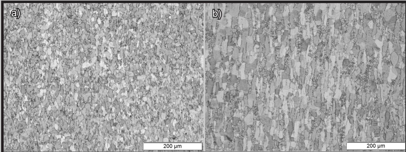
FIG. 1. Optical microscope images of initial microstructure of the titanium alloys: a) Ti6Al4V and b) Ti6Al7Nb.
