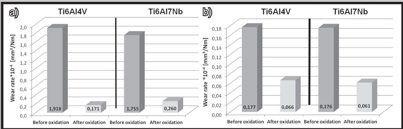
FIG. 4. Wear rates before and after the plasma oxidation of: a) Ti6Al4V and Ti6Al7Nb alloys, b) ZrO<sub>2</sub> countersamples.
