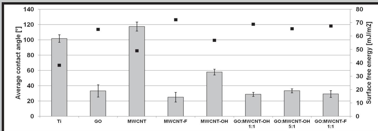
FIG. 9. Contact angles (bars) and average surface free energy (points) values for all deposited coatings.
